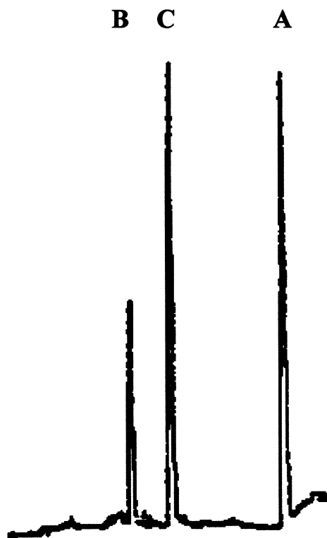
Fig. 2. Electropherogram of compounds A (cimetidine), B and C (migration times 3.99 min, 2.67 min and 3.02 min resp.). Conditions: electrolyte – 10 mM sodium dihydrogenphosphate, pH 3.14, separation voltage 30 kV.
